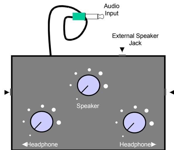
The most expensive component is the volume controls (2 watt x 100 ohm), which are not the same as used in radios and other electronic equipment. If there is interest, this could be a good group project, which would help bring the cost down.
